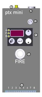
ptx Mini is equipped with an aerial socket  $^{\textcircled{1}}$  and a connector for the battery charger  $^{\textcircled{2}}$  , both at the top of the tool.
