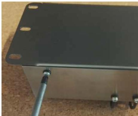
**1) Remove the 6 body fixing screws**
