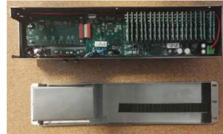
**2) When finished to remove the 6 screws from the BFS, remove the underside of the body by pulling upwards**
